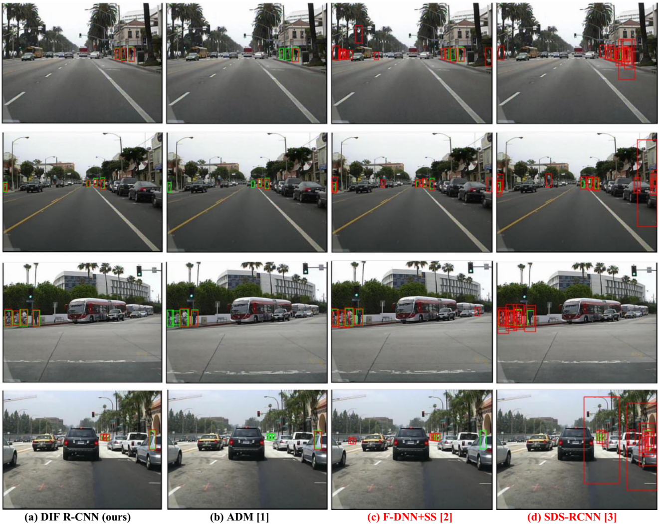
Fig. 8 Visual comparisons of our detection results vs. those of two state-of-the-art methods on the Caltech benchmark. The red bounding boxes show the detection results, and the green bounding boxes denote the ground truth. a DIF R-CNN (ours), b ADM [1], c F-DNN+SS [2], d SDS-RCNN [3]
