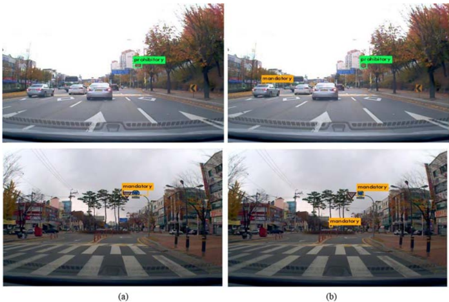
Fig. 7 Detection results comparison of original YOLOv3(left) and optimized YOLOv3(right)
