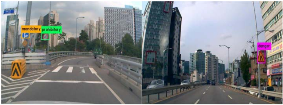
Fig. 2 Experimental detection results of ATSR, on prohibitory, mandatory, and danger class traffic signs
