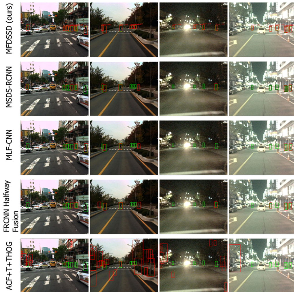
Fig. 9. Visual comparison of our detection results in the KAIST test set with other approaches. The five rows show detection results of MFDSSD (ours) (see Visualization 1), MSDS-RCNN [29], MLF-RCNN [25], FRCNN Halfway Fusion [23], and ACF + T + THOG [21], respectively. The green bounding boxes denote the ground truth. The red bounding boxes show the detection results.
